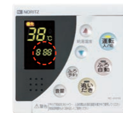
An example of check-up alert: “888” is displayed on the screen (To be fully activated for residential-use equipment only in the Japanese market in 2019.)
